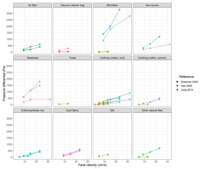
Figure S1. Pressure differential versus face velocity for a single layer of various materials.
